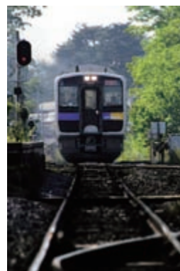
The world's first diesel hybrid railcar Kiha E200 Type
