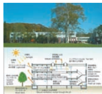
The simple building form, exterior insulation and highly-insulative sash windows
