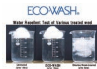
Water repellent test of various treated wool
