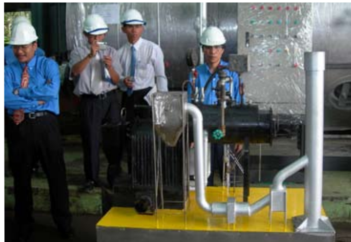
Observing a biomass boiler prototype at M/s Thai K Boiler
