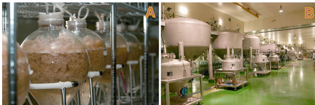
Figure 3. Balloon-type Bubble Bioreactor (A) and Drum-type Bubble Bioreactor (B)
