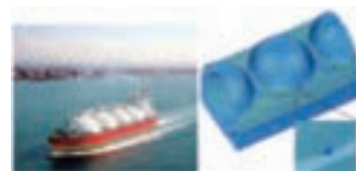
Natural gas carrier ship and the parts where FCA-W is used (from a calculation model used for hull evaluation by Nippon Kaiji Kyokai)
