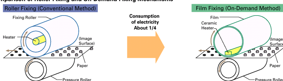
Figure 7 Comparison of Roller Fixing and On-demand Fixing Mechanisms
