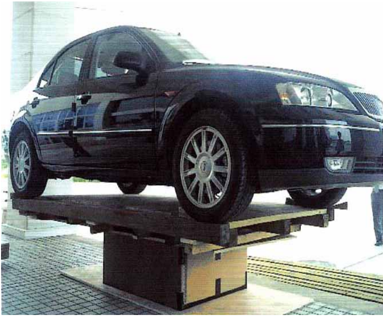
Image 4. Tri-wall's three-layered cardboard supporting an automobile
