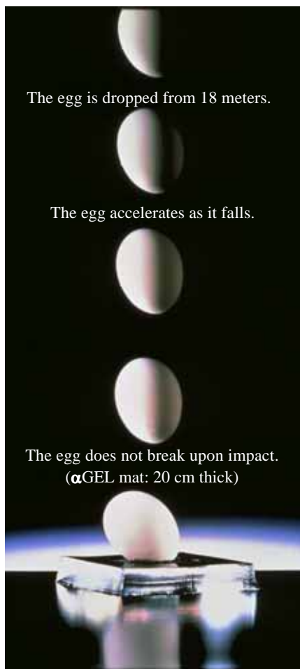
Image 5. αGEL mat cushioning the fall of a raw egg
