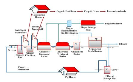
Figure 1. Flowchart of the three-step piggery wastewater treatment (TPWT) system. Source: Su J.J.
