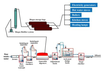
Figure 2. Flowchart of the Three-step Piggery Wastewater Treatment (TPWT) system with a biogas desulfurization biofilter.
