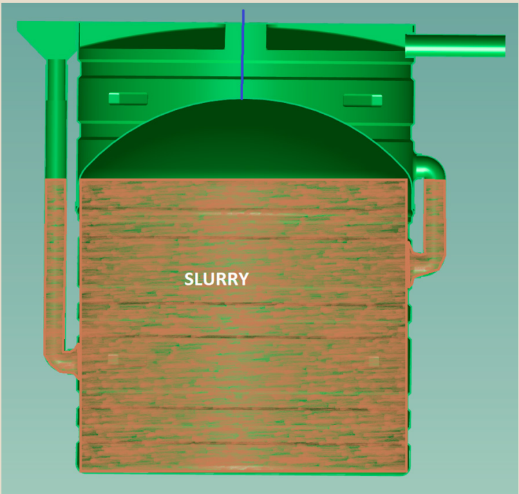
FIGURE 9 SLURRY IS STORED IN THE LOWER DRUM OF AN LLDPE BIODIGESTER (STEP 1).
