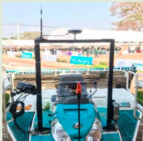
Precision tools attached to a rice transplanter
